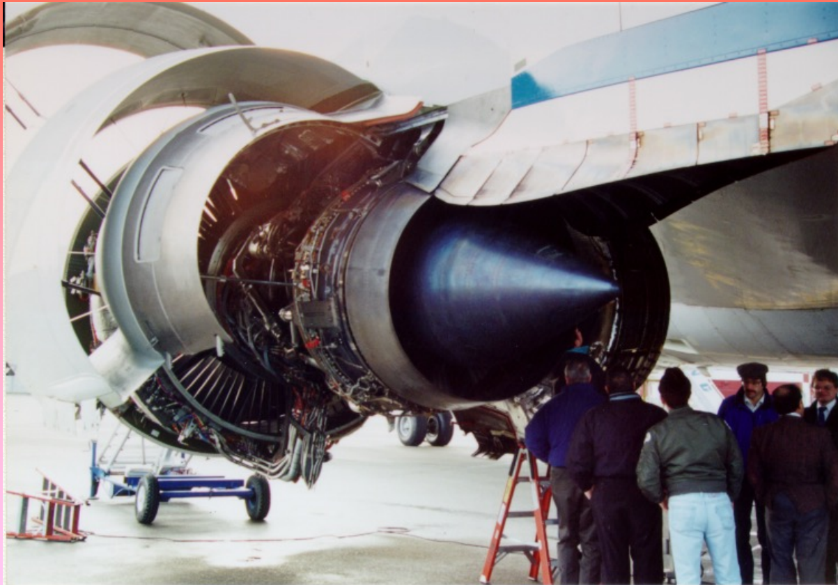
Boeing 777 Plug and Nozzle and Heat Shields
