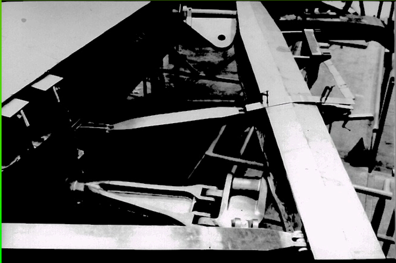
Boeing 757 Mockup - Landing Gear Support Structure
